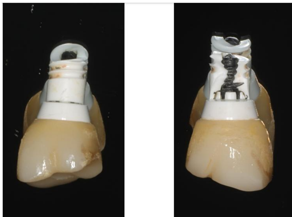
Figure 8: Internal-Implant connection fractographic behavior. (A) Implant fracture propagated radially between the 2 nd and 3 rd threads. (B) Vertical crack propagation exposed the Vicarbo screw and abutment.
